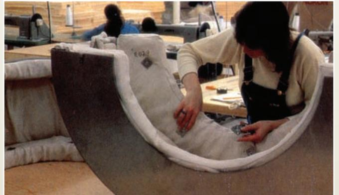
*When specified for added impact and abuse resistance, RE/WRAP insulation components can be supplied with metal jackets having quick release latches to make removal and reinstallation fast and easy. In the case of this component, RE/WRAP insulation blankets have been permanently affixed within the metal jacket; a single operation takes care of removal or reinstallation of both jacket and insulation as one unit.*
